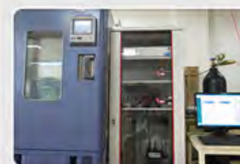
Automatic Pressure Test System
