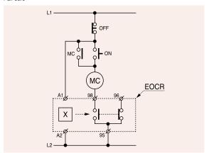
The output of relay is normally energized with control power applied. It is called NVR (No Volt Release) function and recommended to use output mode for safe protection.
